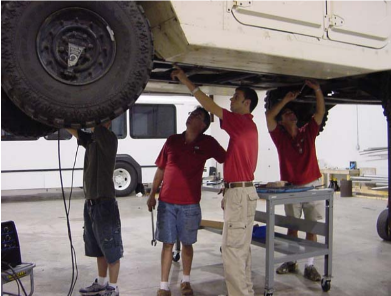
Figure 25: Filter Installation on Hummer Vehicle Platform
