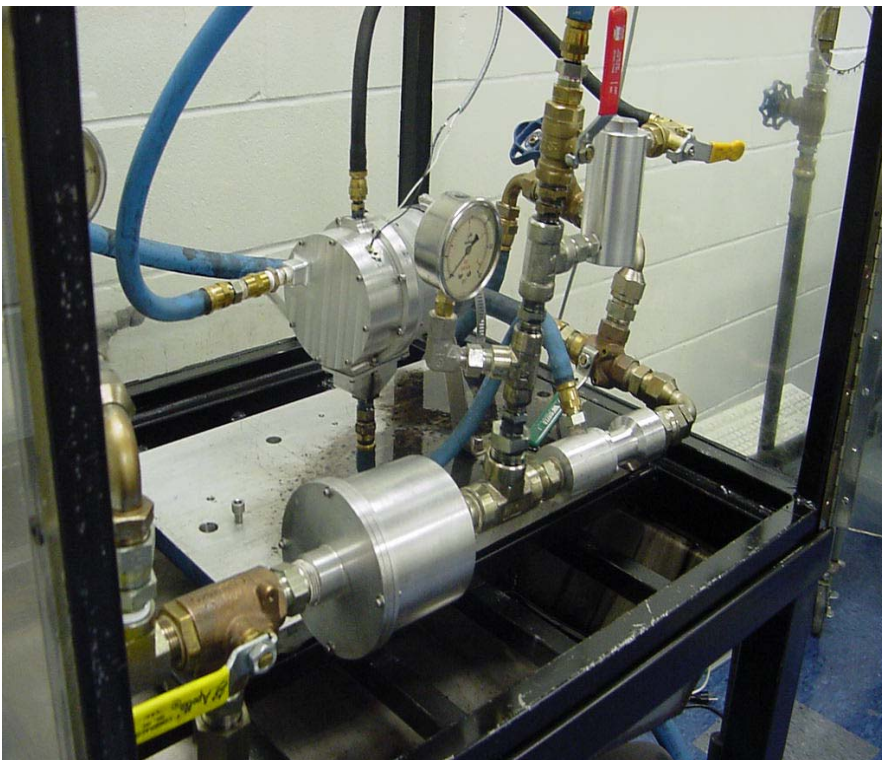
Figure 15: Centrifugal Filter Test Rig
